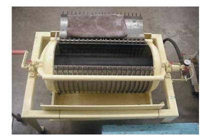
Figure 1.11: Bladder press, 100L capacity.
