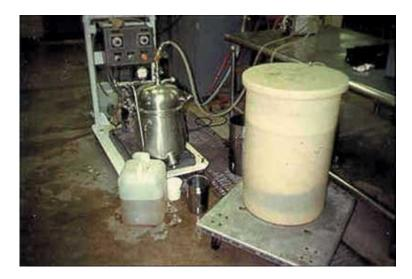
Figure 1.15: Plate and frame and vacuum filter.
