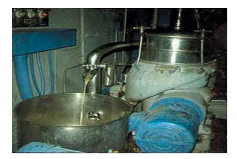
Figure 1.14: Continuous centrifuges. Commercial ~200-1 000 L/hr, Pilot plant ~ 5 to 20 L/hr
