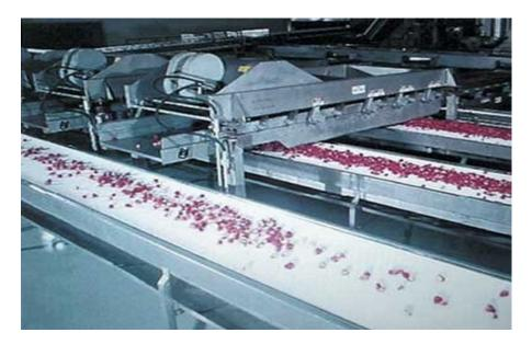
Figure 1.3: Automatic inspection/grading system. Courtesy Key Technology, Inc. (Key, 2000)
