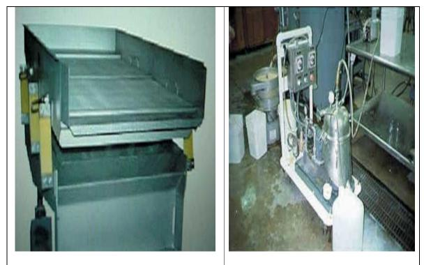
Figure 1.13b: Shaker separating screen used in conjunction with a continuous centrifuge.
