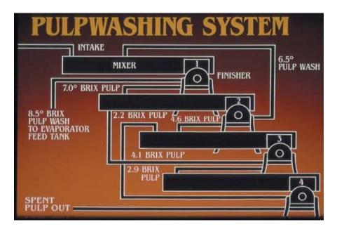
Figure 1.7: Pulp wash extraction schematic.
