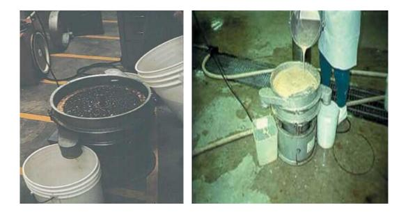
Figure 1.13a: Shaker separating screen. Mesh size and vibration frequency can be varied to accommodate feed viscosity
